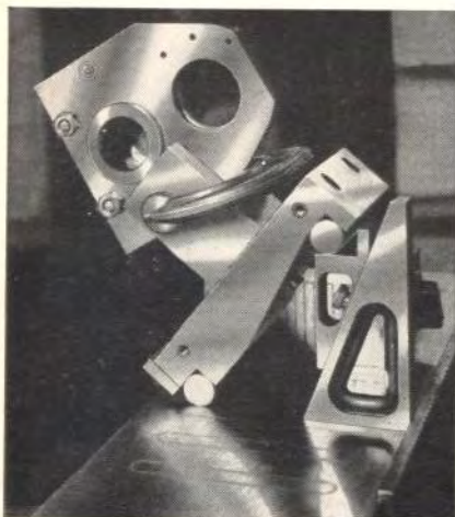
Used in Conjunction with Sine Bar in Grinding Angles
