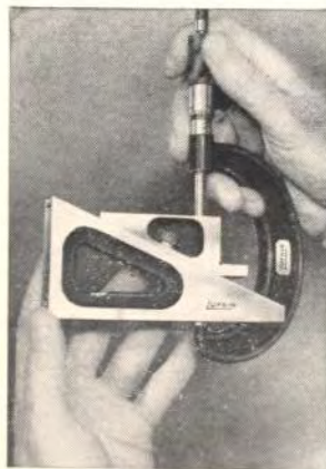
Gage Being Set to Micrometer Accuracy
